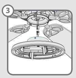
Using the single pin connectors, connect the black or blue wire from the fan to the black wire from the light kit. Connect the white wire from the fan to the white wire from the light kit.
